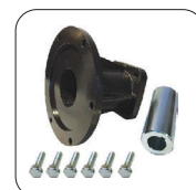
Hydraulic Flange Kit AR55384. For models AR330, AR380, AR410 & AR460 Pumps. Fits SAE 2-Bolt A flange motors with 1" shaft.
