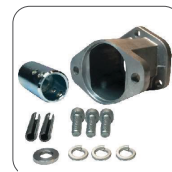
Hydraulic Flange Kit AR43396. For models AR70, AR115, AR135 (SP Models Only). Fits SAE 2-bolt A Flange Motors with 1" Shaft. (Supersedes AR2495).
